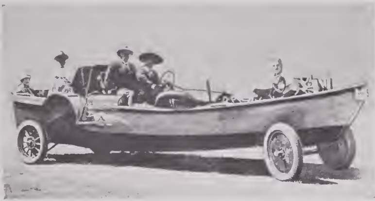
FIGURE 14. Jagger 1926 amphibian using Ford Model T components with chain drive to rear wheels and removable paddle wheels for water propulsion. Water speed about 4 mph.
